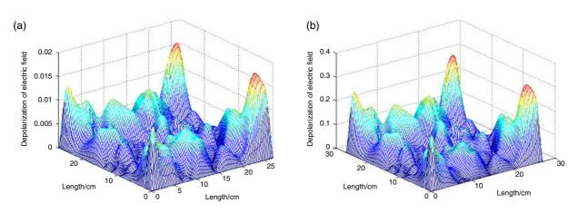
Figure 7. The depolarization of the laser passing through (a) one disk and (b) twenty disks.
