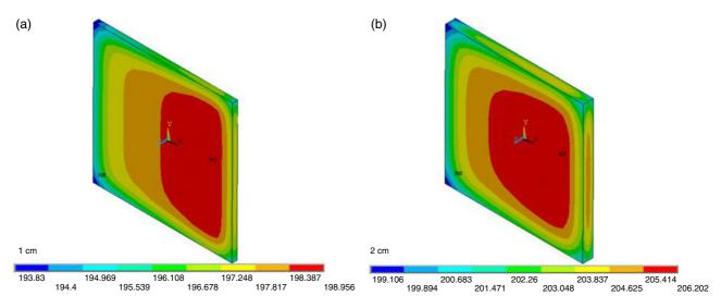
Figure 1. Temperature distribution of Yb:YAG: (a) temperature of 1 cm Yb:YAG; (b) temperature of 2 cm Yb:YAG.
