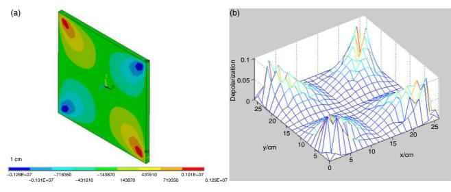
Figure 2. (a) xy shear stress of Yb:YAG; (b) depolarization of one disk.
