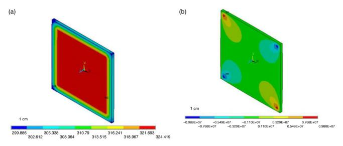
Figure 3. (a) Temperature distribution and (b) xy shear stress of Nd:glass.
