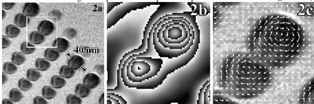
Fig.2 The in-focus image of 2D-array of Ni-nanodots grown on amorphous carbon membrane and viewed in Fresnel Lorentz mode (2a). The size of each nanodot is about 40 nm. Fig. 2b shows the equipotential contours of the reconstructed phase for the boxed area highlighted in (2a). The phase gradient information as M-vector map (magnetization) is shown in Fig. 2c.
