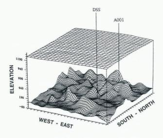
Fig. 2. "Wire mesh" view of the bedrock and ice surface around Law Dome summit. The survey grid is  $15 \, \mathrm{km} \times 15 \, \mathrm{km}$ , and the bedrock is exaggerated in the vertical by five times. The surface ice velocity is zero near (just north of) the highest point on the dome, A001.
