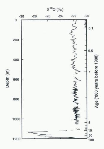
Fig. 7. Oxygen-isotope ratio profile for DSS ice core. The top 391 m is from smoothed fine-detail (~10 per year) measurements. The 391–1000 m section comprises 0.5 m contiguous samples. The transition, LGM and Wisconsinan, is from spot samples, and the basal ice is sections with measurements at 10 mm intervals.
