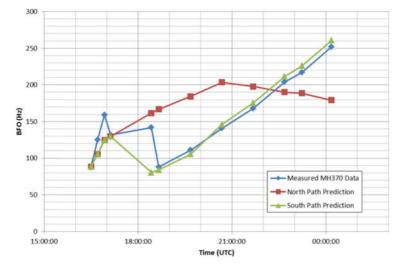
Figure 14. BFO Results using Refined Model.
