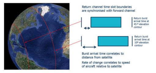
Figure 1. Burst Time Offset Principle.
