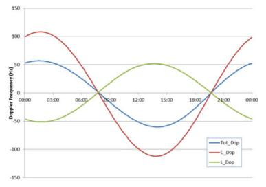
Figure 10. Calculated Pilot Frequency Doppler Offset.
