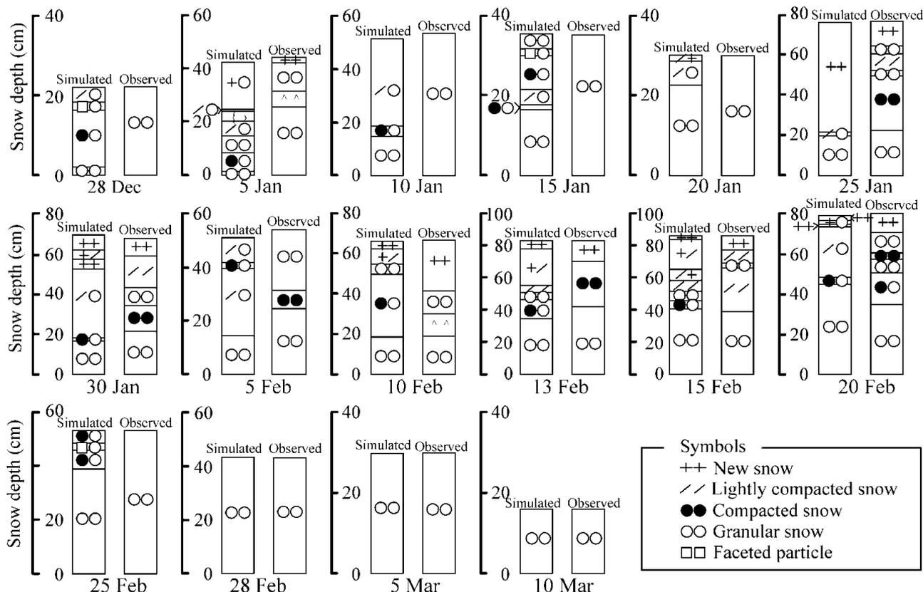
Fig. 4. Comparisons between snow-type measurement and simulations in 2001/02 at NISIS.
