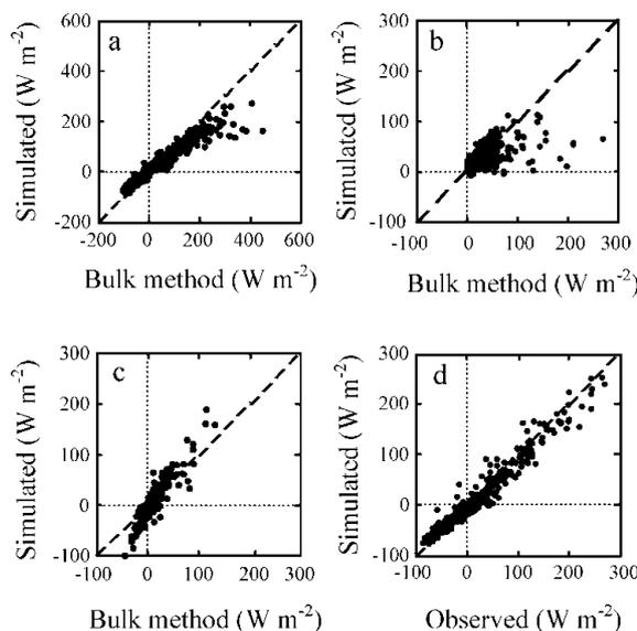
Fig. 8. Comparisons between bulk method and simulation in 2001/02 at NISIS. Net radiation was measured directly. (a) Energy balance at surface; (b) sensible-heat flux; (c) latent-heat flux; (d) net radiation.
