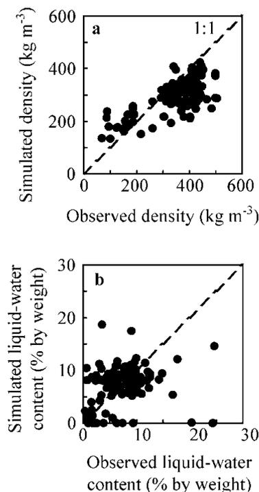
Fig. 5. Comparisons between measurement and simulation in 2001/02 at NISIS: (a) density; (b) liquid-water content.
