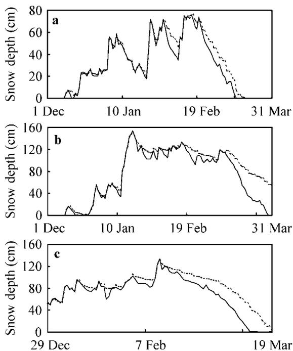
Fig. 1. Comparisons between snow-depth measurements and simulations. Solid lines indicate measurement, and dashed lines indicate simulation. (a) NISIS in 2001/02; (b) NISIS in 2000/01; (c) SB in 2001/02.
