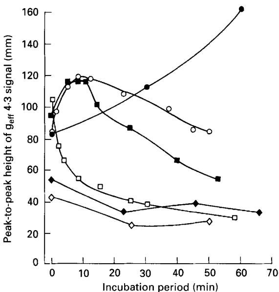
Fig. 7. Electron paramagnetic resonance (EPR) variables of Fe-ascorbate solutions. Experiments performed as in Fig. 6. Background corrected peak-to-peak height of  $g_{\text{eff}}$  4-3 (0.17 T) signal in spectra as a function of incubation time at 37°. Samples were initially air-equilibrated (□, ■, ○, ●) or bubbled with nitrogen (◇, ◆). During the incubation sample pH was 6.8 (●, ◆), 7.0 (○), 7.2 (■) or 7.4 (□, ◇).
