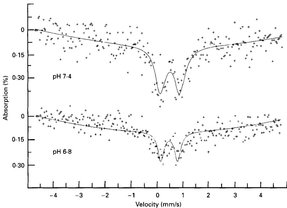
Fig. 8. The 77 K Mössbauer spectra of  $^{57}\text{Fe}$ -ascorbate solutions prepared as described in Fig. 1 at pH 6.8 and 7.4. Incubation was for 1 h at  $37^\circ$ , then samples were frozen for analysis.
