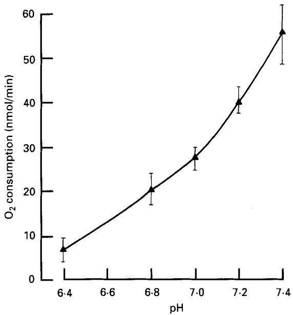
Fig. 9. Oxygen consumption by iron-ascorbate solutions. media were prepared, incubated at  $37^\circ$  and initial rate of O<sub>2</sub> consumption measured as described on pp. 158–159. Medium pH was varied and determined in solutions after O<sub>2</sub> consumption determination; Fe concentration was 100  $\mu\text{mol/l}$ , ascorbate 2 mmol/l.
