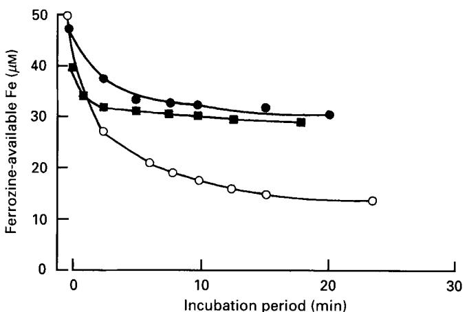
Fig. 4. Effect of medium ascorbate concentrations on rapidly ferrozine-available iron in Fe-ascorbate solutions. Ascorbate concentrations were (mmol/l): 1 (○), 5 (■), 10 (●). For details of procedures, see p. 158 and Fig. 1.
