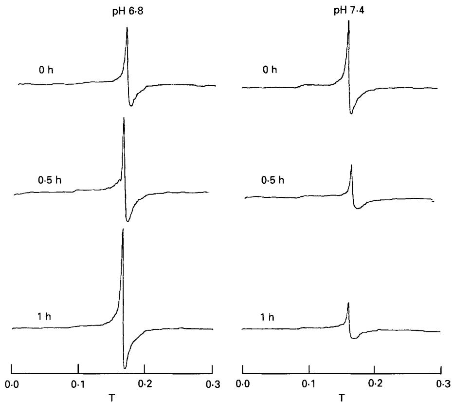
Fig. 6. Electron paramagnetic resonance (EPR) spectra of  $\text{FeCl}_3$ -ascorbate (1:20, v/v) solutions. Fe-ascorbate samples, 0.3 ml (in EPR tubes) were prepared as in Fig. 1, incubated at  $37^\circ$  and frozen at the times indicated. Spectrometer settings were microwave frequency 9.11 GHz, microwave power 20 mW, 100 kHz modulation, modulation amplitude 8, sweep time 32 min, temperature 103 K, time constant 0.3 s.
