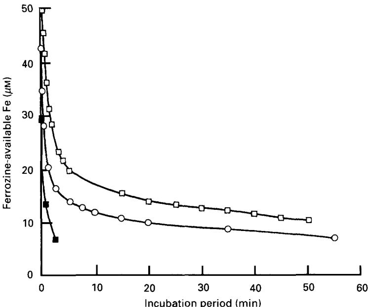
Fig. 3. Effect of medium composition on loss of ferrozine-available iron from Fe-ascorbate solutions. Rapidly ferrozine-chelatable Fe was determined as shown in Fig. 2 (pH 7.4) in Fe-ascorbate solutions shown in Fig. 2 (□) or lacking mannitol (■) or lacking NaCl (○). For details of procedures, see p. 158.
