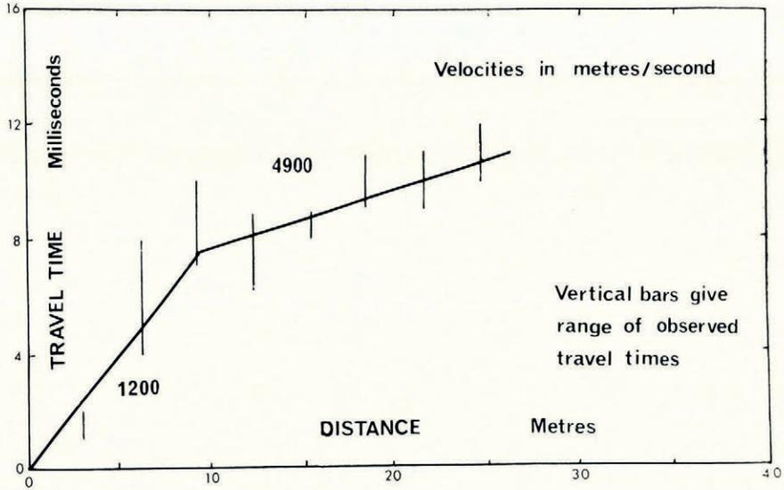
Fig. 4. Seismic travel-time data, Taylor Valley, on exfoliated granite at an altitude of 150 m. above Lake Bonney
