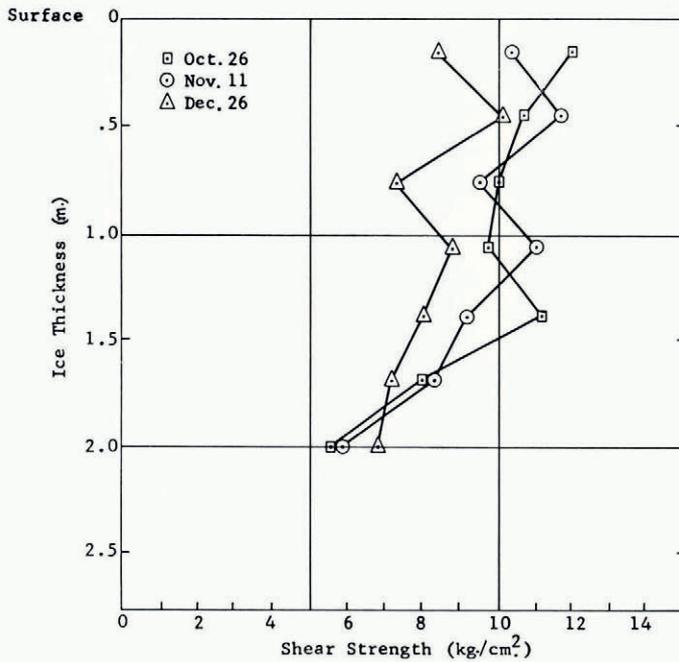
Fig. 6. Shear-strength profile of the sea-ice sheet on 26 October, 11 November and 26 December 1964
