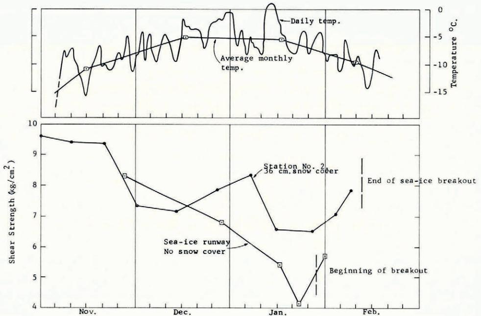
Fig. 14. Average shear strength of the sea-ice sheet compared with temperature and time
