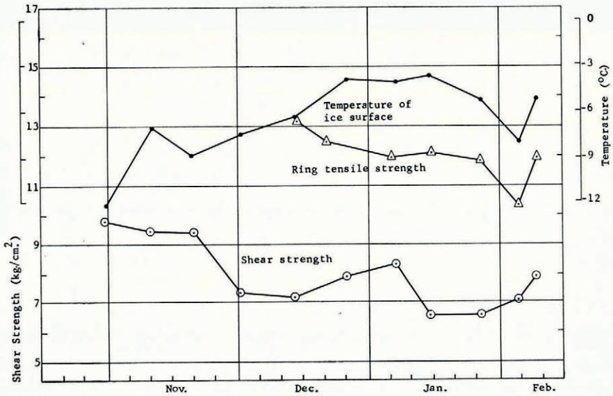
Fig. 7. Average shear and ring-tensile strengths of the sea-ice sheet compared with ice-surface temperature and time. NCEL station No. 2
