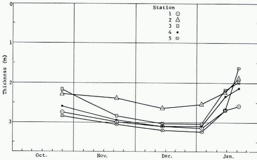
Fig. 9. Ice-thickness changes during the summer of "Deep Freeze 65". NCEL stations 1 to 5
