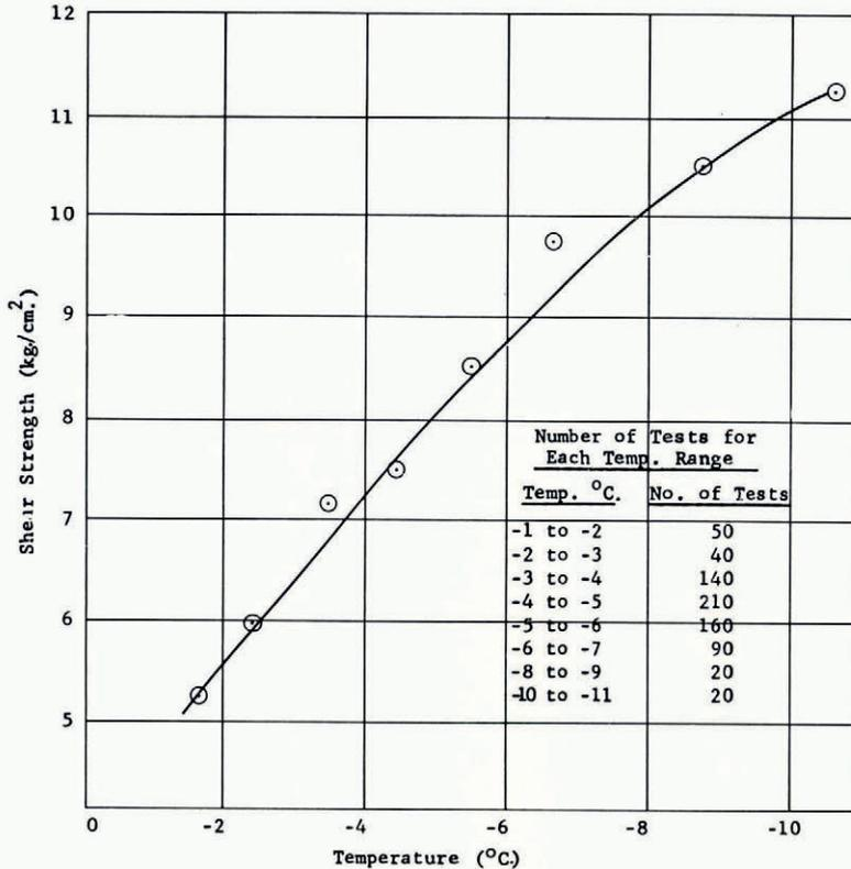
Fig. 3. Average shear strength of sea ice as a function of temperature. NCEL station No. 2
