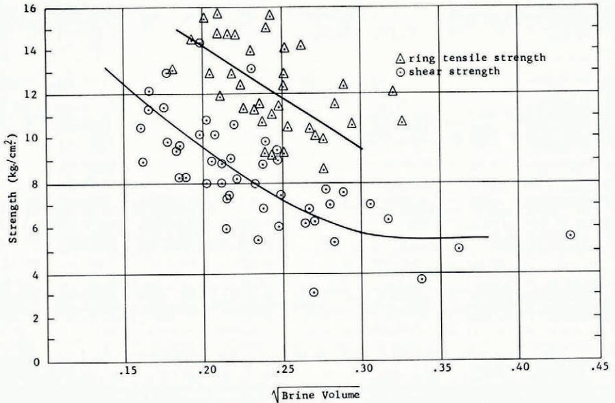
Fig. 8. Shear and ring-tensile strengths as a function of brine volume
