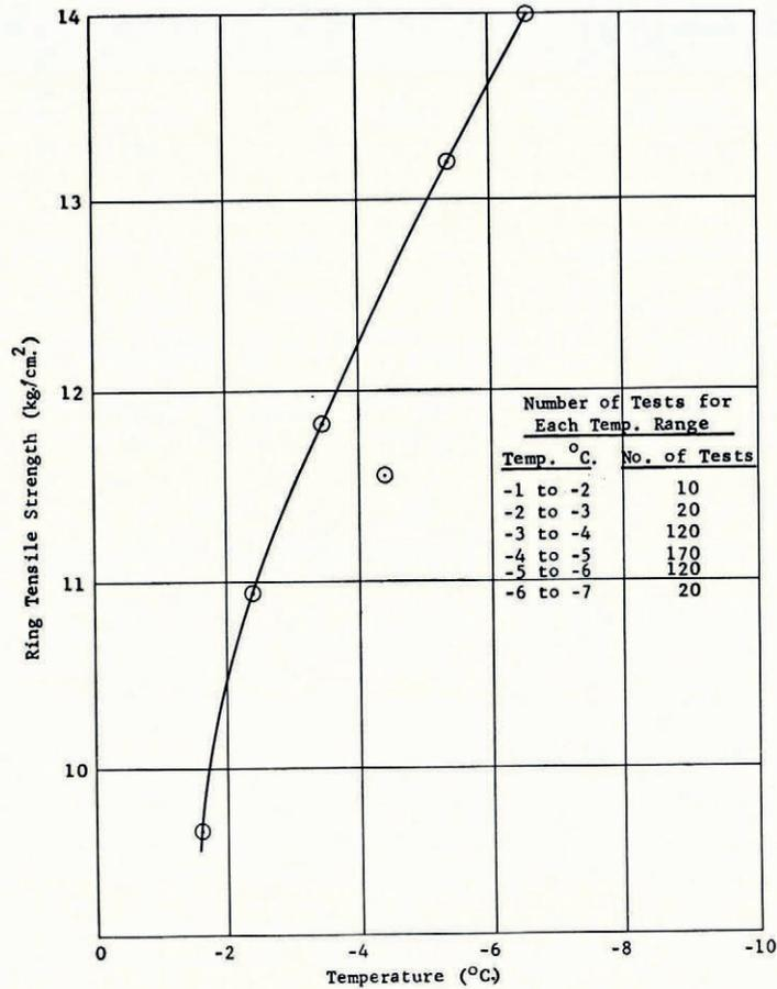
Fig. 4. Average ring-tensile strength of sea ice as a function of temperature. NCEL station No. 2
