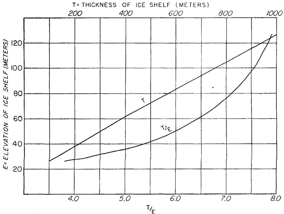
Fig. 5. Relationship of surface elevation and ice thickness for a floating ice shelf based on the density-depth data from the SIPRE deep bore-hole at Little America V
