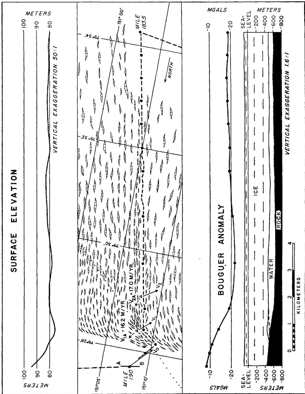
Fig. 3. Geophysical studies at "Fashion Lane": (a) elevation profile; (b) crevasse pattern; (c) movement studies; (d) ice thickness determinations; (e) rock topography
