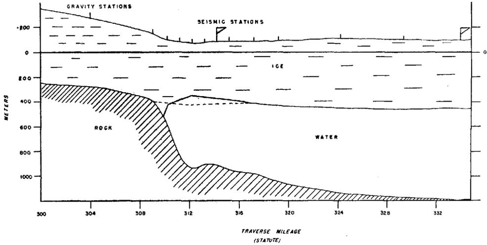
Fig. 4. Contact of Filchner Ice Shelf and grounded ice at lat.  $80^{\circ} 36' 4''$  S., long.  $46^{\circ} 59' 0''$  W. The bottom of the shelf near the contact is drawn (1) assuming complete and local hydrostatic equilibrium and (2) a uniform shelf thickness
