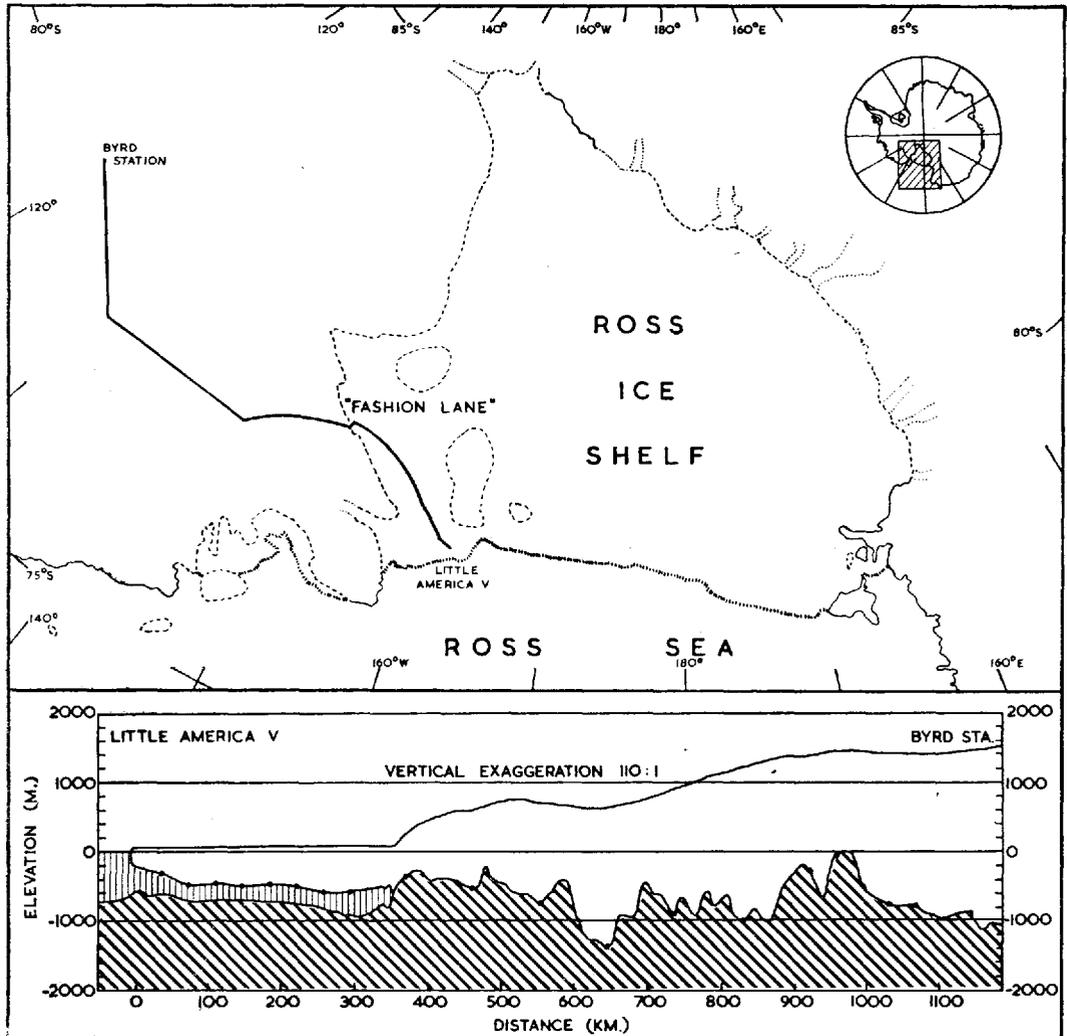
Fig. 1. Profile of ice thickness and bedrock topography along Army-Navy trail from Little America V to Byrd Station
