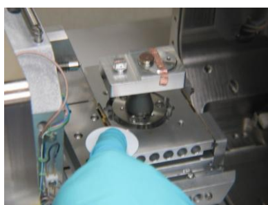
Figure 3. The FIB stage survey, conducted upon loading and unloading of the specimen.
