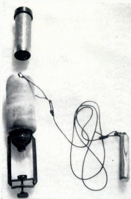
Fig. 1. Centrifuge for separating water from melting snow (see E. R. LaChapelle, p. 769)
