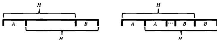
Having isolated  $A$  as a head string of  $S$  (left-hand diagram), it is also a head string of  $H$  (right-hand diagram), and the same applies to  $B$  as a tail. This reasoning iterates.
