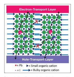
Schematic for a 2D perovskite in which the metal-halide frameworks are flipped on their ends and oriented perpendicular to the substrate. The photo-generated charges can pass uninterruptedly through the vertical columns formed by the metal-halide framework.
