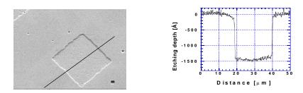
Fig.4: SEM and profilometer scan of ion implanted and etched GaN
