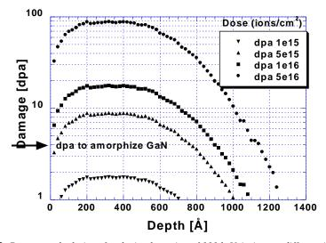
**Fig.2**: Damage calculations for the implantation of 100 keV Ar ions at different ion doses. The dpa to amorphize GaN is the approximate threshold from references [11] and [13].
