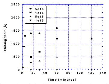
**Fig.1**: Dependence of etching depth on etching time for the implantation of 100 keV Ar ions at different ion doses.
