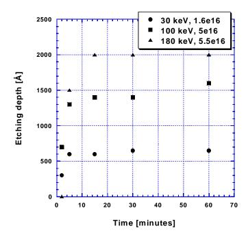
Fig.3: Dependence of etching depth on etching time for different Ar ion energies.
