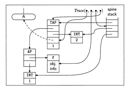
Fig. 11. The reduction of a traced redex f 1 2. The figure illustrates the situation just before *Trace* is called from the code for f.
