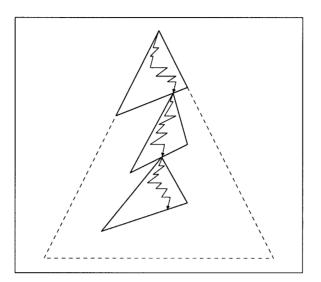
Fig. 6. Piecemeal EDT generation. The large, dashed triangle represents the entire EDT, the smaller triangles represent the parts of the EDT which are stored during the first, second and third execution. The path going from the root downwards illustrates how the EDT is traversed during debugging.
