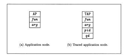
Fig. 9. The layout of untraced and traced application nodes. AP and TAP are the node tags. The fields fun and arg are pointers to the applied function and the argument, respectively. The field *pid* is the identity of the parent, and *qd*, finally, is the estimated query distance.
