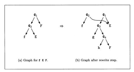
Fig. 3. Graph reduction of f E F. The application node indices identify physical heap locations.
