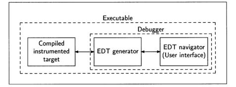
Fig. 7. The components of a debuggable executable. The target program has been compiled for debugging, resulting in instrumented object code. This is linked with the EDT generator and the EDT navigator thus forming a debuggable executable.
