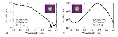
Figure 4. SWIR wing of SC spectra under optimal excitation conditions in YAG crystals: (a) 15 mm and (b) 130 mm long. The insets show the corresponding beam profiles.
