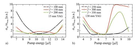
**Figure 3.** Ratio of the energy stability of the SC and the pump pulse  $\sigma_{SC}/\sigma_{Pump}$  as a function of the pump energy for different focusing into YAG crystals: (a) 15 mm and (b) 130 mm.
