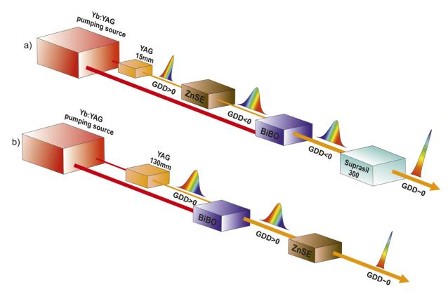
Figure 5. Single-stage OPCPA configurations with (a) short and (b) long YAG crystals for SC generation.
