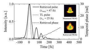
**Figure 7.** SHG-FROG retrieved temporal profile (solid line) and temporal phase (dashed line) of an amplified signal pulse after compression in Suprasil 300 with SC seed from a 15 mm YAG crystal compared to a transform-limited pulse calculated from the measured spectrum (dotted line).  $\tau_{TL}$ , transform-limited pulse width. Insets, measured (top) and reconstructed (bottom) FROG traces with an error of 0.9% using a grid of 512 × 512 points.
