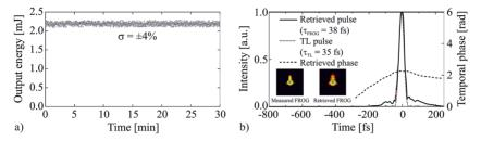
**Figure 9.** (a) Amplified output energy stability of the OPCPA system for 30 min of operation. (b) SHG-FROG retrieved temporal profile (solid line) and temporal phase (dashed line) of the compressed signal pulse at maximum output energy compared to the transform-limited pulse calculated from the measured spectrum (dotted line).  $\tau_{TL}$ , transform-limited pulse width. Insets, measured (top) and reconstructed (bottom) FROG traces with an error of 1.1% using a grid of 512 × 512 points.
