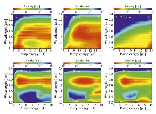
Figure 2. Dependence of the intensity of the SC spectrum envelope on the pump pulse energy at different focal lengths for YAG crystals 15 mm (a)–(c) and 130 mm (d)–(f).
