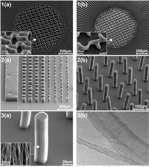
**Fig. 1(a)** and **Fig. 1(b)** demonstrate the complexity of patterns attainable with the reported CVD process. The insets in each case are magnified images of the MWCNT growth.
