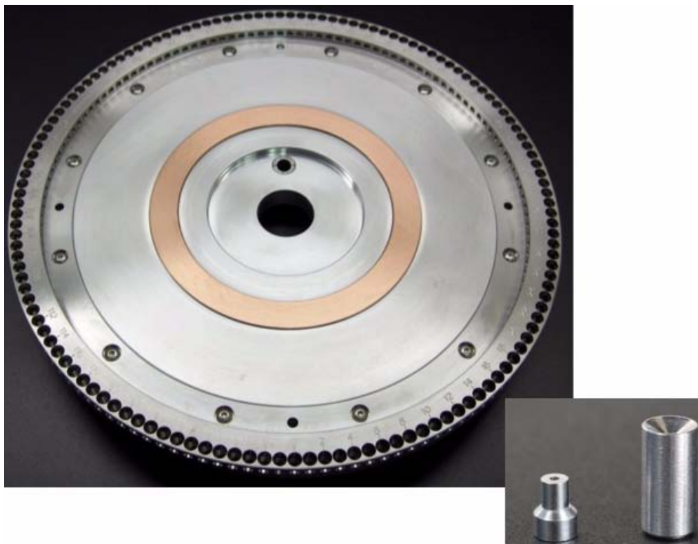
Figure 2 The 134-sample wheel. The lower insert shows our new front-loading sample holders (right) compared to the NEC sample holders (left).
