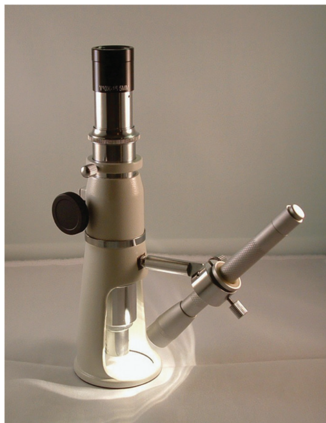
Figure 1: The typical shop inspection microscope. The flashlight on the extension arm is adjustable and both are easily removed.
