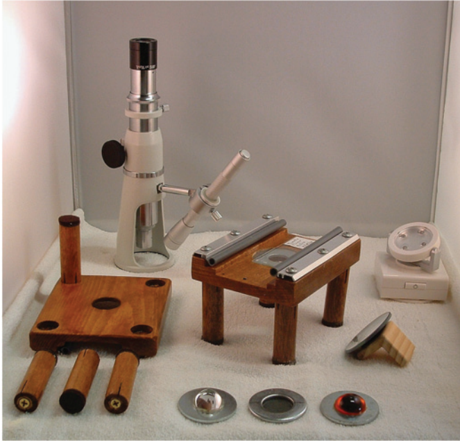
Figure 4: Shop inspection microscope and platform stage with a few accessories: sub-stage condenser, polarizing filter, Rheinberg darkfield filter, and sub-stage mirror.
