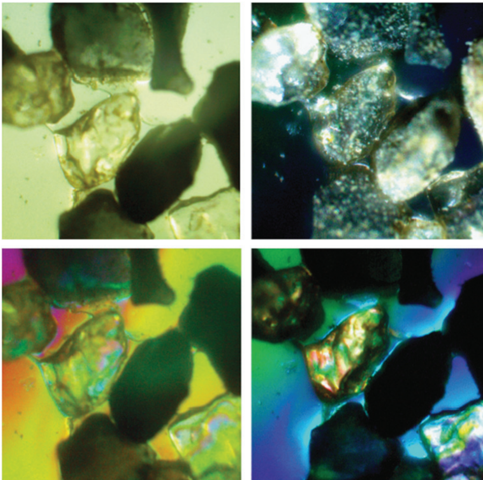
Figure 8: Example images of sand grains from Wyoming taken with the shop-inspection field microscope. Clockwise from upper left: sub-stage transmitted light, oblique epi-illumination, cross-polarized light, cross-polarized light with wave plate (cellophane wrap). All images were taken with an Amscope eyepiece camera and 10× objective. Image width = 1.0 mm.
