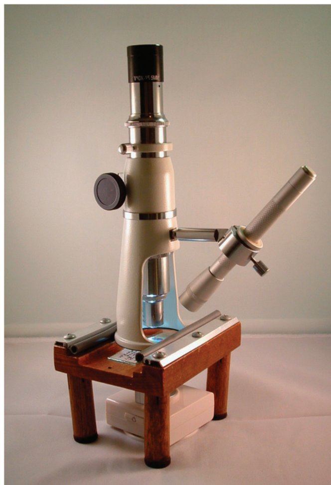
Figure 3: Do-it-yourself platform stage for the shop inspection microscope.
