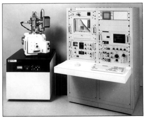
Focused Ion Beam Milling System
