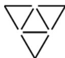
Fig. 7. Decomposition of the initial shape C of the shape grammar of triangles into six atoms.
