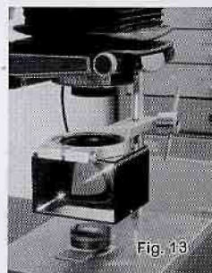
Figure 13-Olympus PM-EL80 vertical illuminator mounted in a stand above a metallographic specimen.
