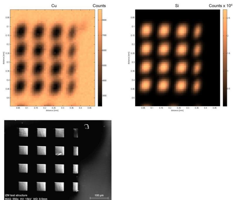
**Figure 2.** XRF Maps of Cu Kα and Si Kα (top left and top right), compared to the picture generated by the detection of secondary electrons.
