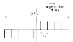
Fig. 5. The convolution function with the required spatial frequency response to restore a dual-beam observation to the equivalent single-beam observation.
