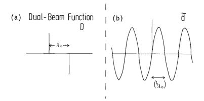
Fig. 1. (a) The dual-beam function, and (b) a representation of its Fourier transform.  $\lambda_0$  is the angular separation of the 2 far-field beams.
