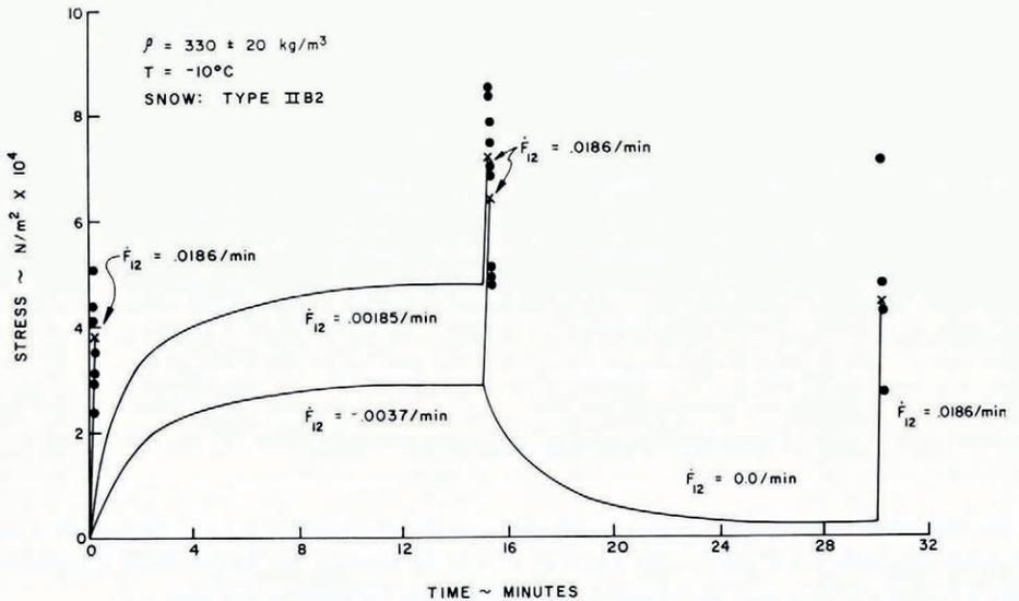
Fig. 3. Comparison of fracture criterion with experimental results for shear.
