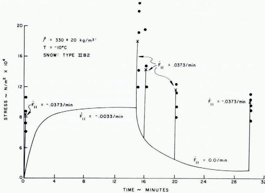
Fig. 1. Comparison of fracture criterion with experimental results for unconfined compression.
