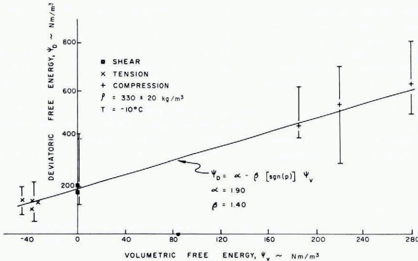
Fig. 4. Comparison of fracture criterion with experimental results for brittle fracture conditions.
