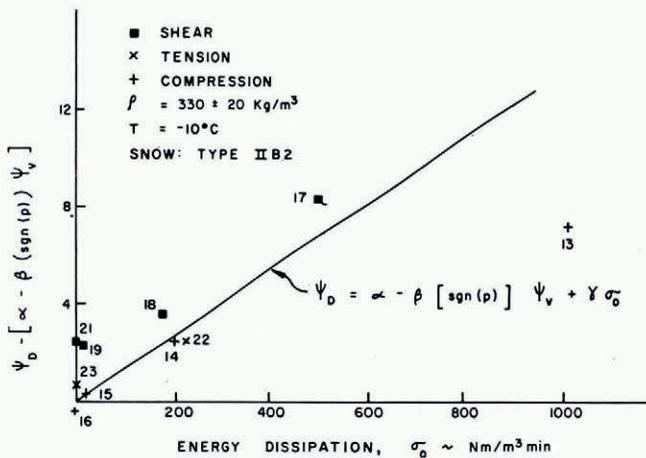
Fig. 5. Comparison of fracture criterion with experimental results for ductile fracture conditions.
