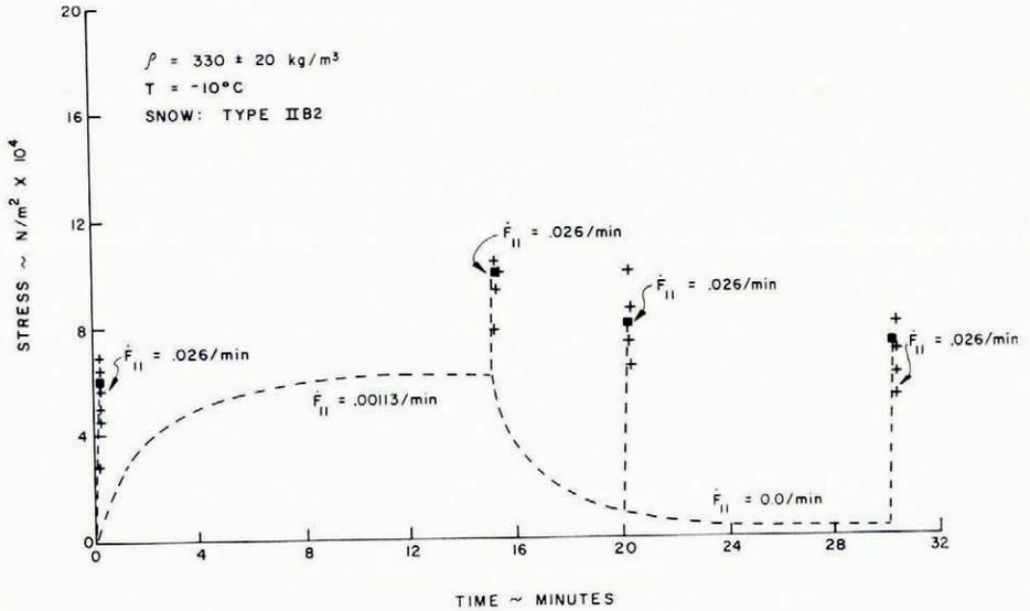
Fig. 2. Comparison of fracture criterion with experimental results for tension.
