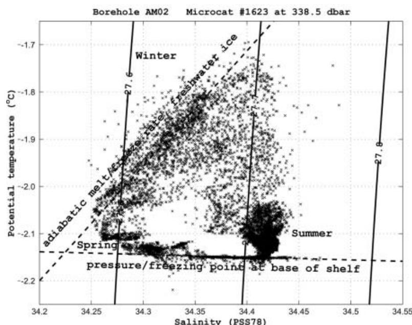
**Fig. 6.** Potential-temperature vs salinity diagram for 2001 from the upper CTD instrument ( $P=338$  dbar) at the AM02 site. Water-mass characteristics show seasonal variability which follows an anticlockwise cycle in ( $\theta$ - $S$ ) space.
