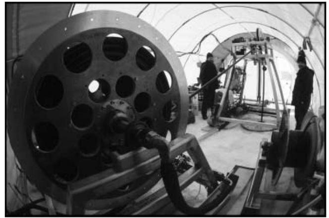
**Fig. 2.** Set-up of the AMISOR HWD drill tent with hose winch in left foreground and capstan stand over the borehole in right background.
