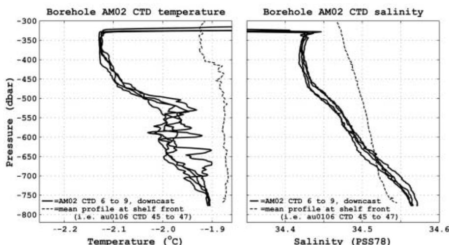
**Fig. 4.** CTD data profiles in the 468 m deep ocean cavity beneath the ice shelf at AM02, January 2001. Also shown is a representative mean profile (dashed line) at equivalent depths in the water column out front of the shelf (measured 4 weeks later).
