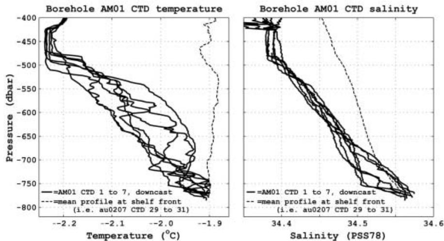
**Fig. 5.** CTD data profiles in the 362 m deep ocean cavity beneath the ice shelf at AM01, January 2002. Also shown is a representative mean profile (dashed line) at equivalent depths in the water column out front of the shelf (measured 2 weeks later).
