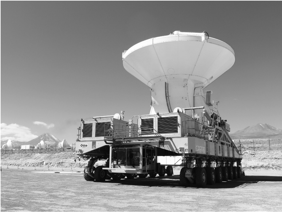
Figure 9.3 ALMA antenna transporter Otto carrying the last antenna, built by AEM, to the high site to join the array. Credit: ESO, CC BY 4.0.
