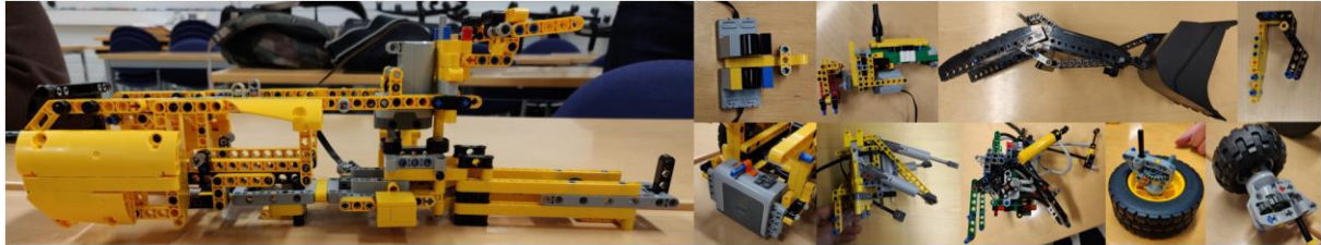
Figure 6. Wheel loader frame based on the FBE partitioning type and the module variants
