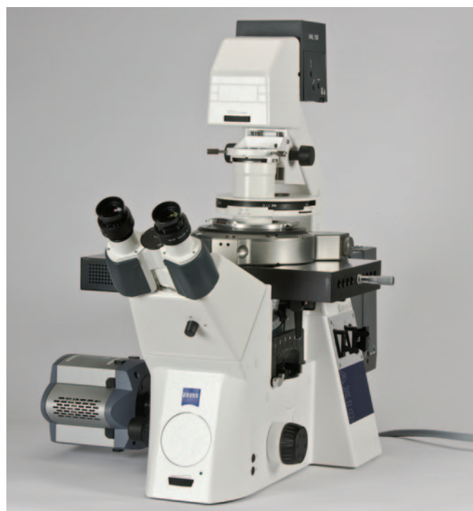
Figure 1: An example of an AFM that was designed specifically for combined ILM-AFM studies; the Agilent 6000ILM AFM mounted on a Zeiss D1 ILM.
