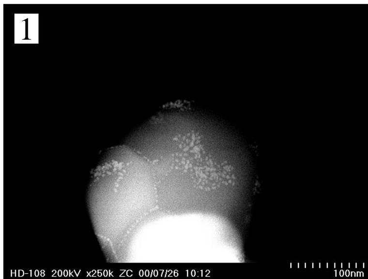
FIG. 1. Z-contrast image of Au nanocrystals deposited on a TiO<sub>2</sub> support from a 0.39 mg/ml Au toluene suspension. The Au deposits both on the facets of the TiO<sub>2</sub> and in the boundaries between crystals.
