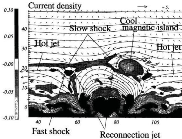
**Figure 2.** Two-dimensional model of reconnection and jet launching as a result of flux emergence from the solar interior. The emerged magnetized plasma collides with the overlying ambient coronal field and a current sheet is formed. Two hot jets are launched sideways along the coronal field lines. A thick plasmoid (cool island) is being formed in the current sheet. From Yokoyama & Shibata (1996)
