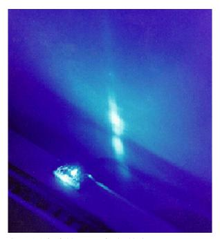
Figure 5. A far-field pattern of pulsed lasing.
