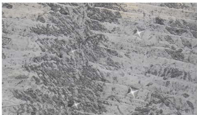
Fig.2- Micrograph of a austenitic-martensitic weld metal structure (500X) Microhardness martensite(dark) 430..460 HV, austenite (light) 230..240 HV
