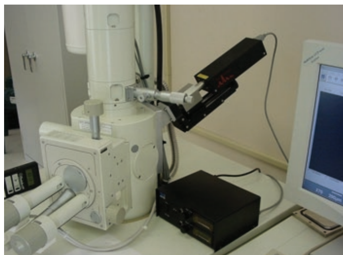
Figure 1: Small-spot fX^{\text{TM}} X-ray tube, producing a spot size of 0.5–5 mm on the sample, attached to an SEM.
