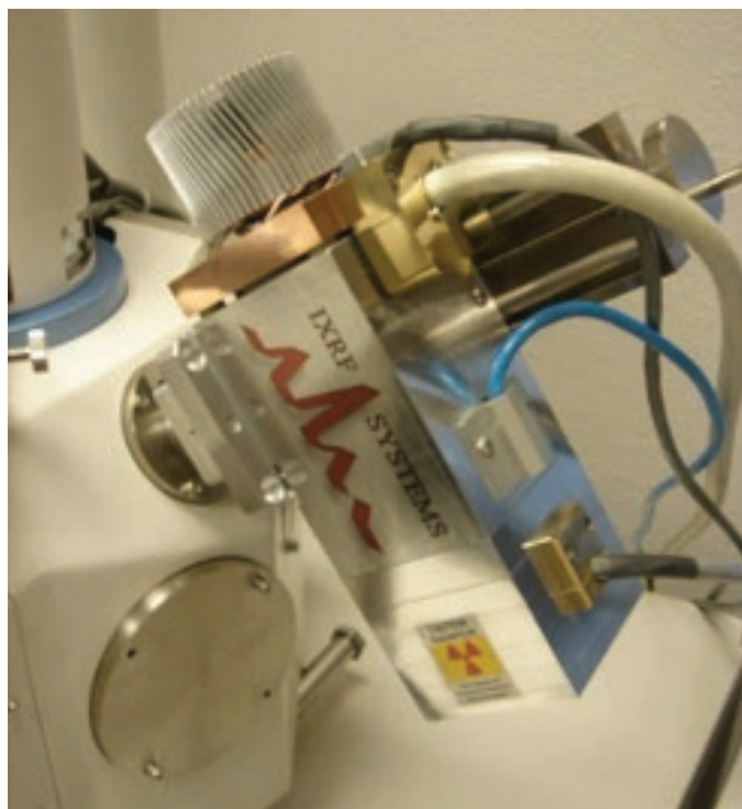
Figure 3: X-Beam™ X-ray source with a polycapillary focusing optic shown attached to an SEM.
