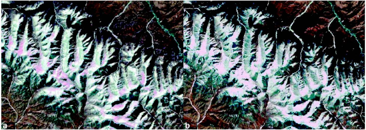
Fig. 6. RGB color composite of ETM+ bands 4, 3 and 2 of the study area (a) after topographic normalization, and (b) without topographic normalization.
