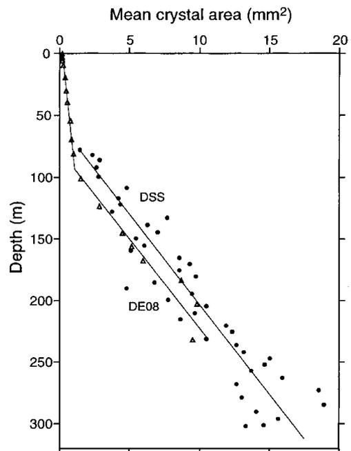
Fig. 1. Plot of crystal size as a function of depth at DE08 (triangles) and DSS (filled circles).
