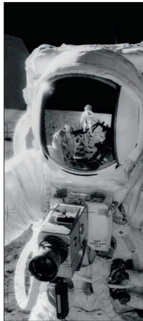
Left: Photo of Apollo 12 extravehicular activity. Alan L. Bean is shown collecting lunar soil samples, while Commander Charles Conrad Jr. is reflected in his helmet visor. Constructed by Air Lock, Inc., the pressure helmet consisted of a high-strength polycarbonate resin, Lexan. Credit: NASA.
