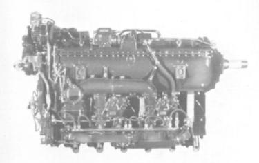
A modern unsupercharged six-cylinder engine of 250 b.h.p., specially developed for the highest reliability and economy in training and light transport service; now in full quantity production and already in large-scale operation between wide extremes of climate
