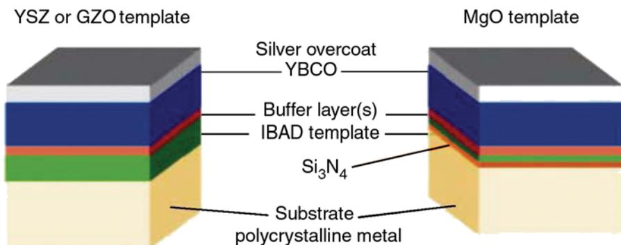
Figure 2. Schematic illustration of the ion-beam-assisted deposition (IBAD) process for fabricating YBCO superconducting wires using yttrium-stabilized zirconia (YSZ),  $Gd_2Zr_2O_7$  (GZO), or MgO template architectures.
