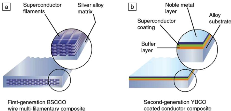
Figure 1. Schematic illustrations of (a) first-generation and (b) second-generation high-temperature superconducting (HTS) wire architectures.
