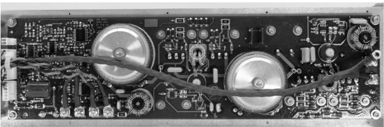
Fig. 8. Assembled motor power supply. The MPS makes use of a number of custom-designed magnetic components to maximize power density. The switching devices, MOSFETs, are located beneath the circuit board.
