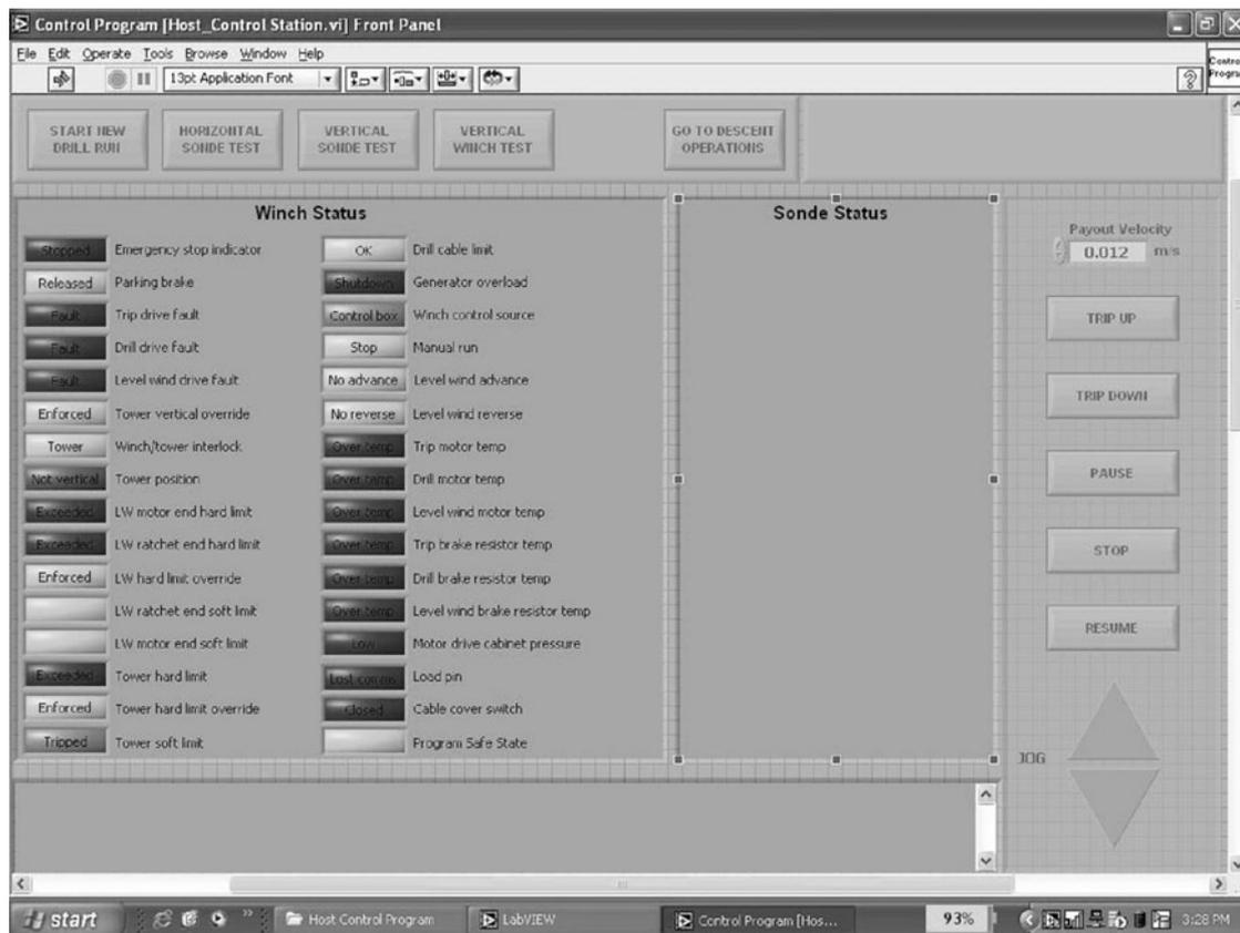
**Fig. 1.** Winch control screen. A number of control lights inform the operator of problems with the system. Winching speed is adjusted by entering desired speed into a data field. Direction is determined by 'Up' and 'Down' buttons. Depending on the state of the drilling action (ascent, descent, coring, etc.) the winch screen changes appearance accordingly.
