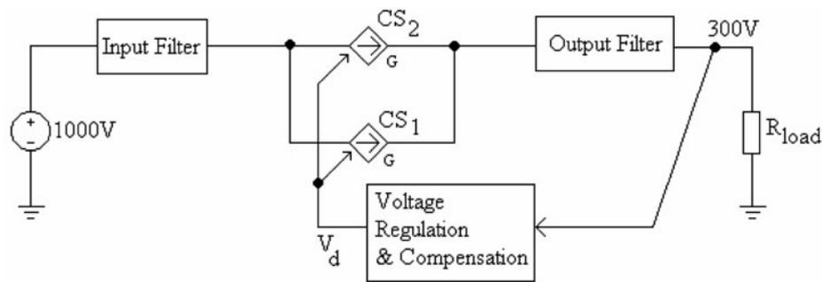
**Fig. 7.** Simplified MPS operating principle. Two voltage-controlled current sources are operated in parallel. A voltage loop ensures constant output voltage over the load range of 0–5 kW. Input and output filters provide low-noise power buses.
