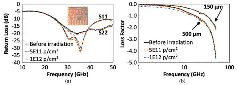
**Fig. 4.** Return loss of two bowtie slot antennas with various circuitry environments. Inset the photograph of the circuitry. Loss factor measured for two CPW lengths (100 and 500 μm) versus frequency.
