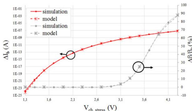
**Fig. 5.** Comparison of simulated  $\Delta I_b$  and  $\Delta\beta/\beta_0$  as a function of  $V_{cb\_stress}$  based on MM degradation model (high-voltage SiGe NPN: after 10 years of stress at 40 °C).
