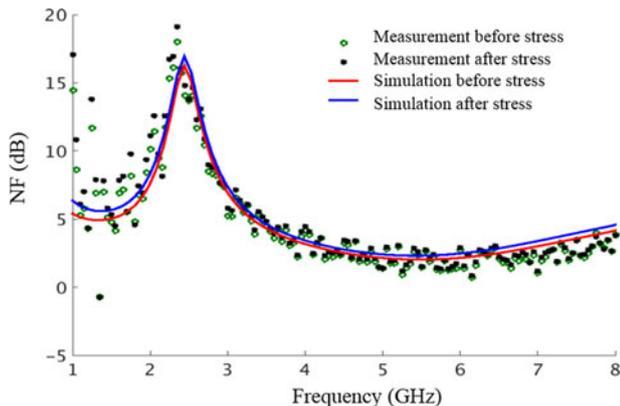
**Fig. 11.** Comparison between simulated and measured NF after 336 h of 20 dBm stress.
