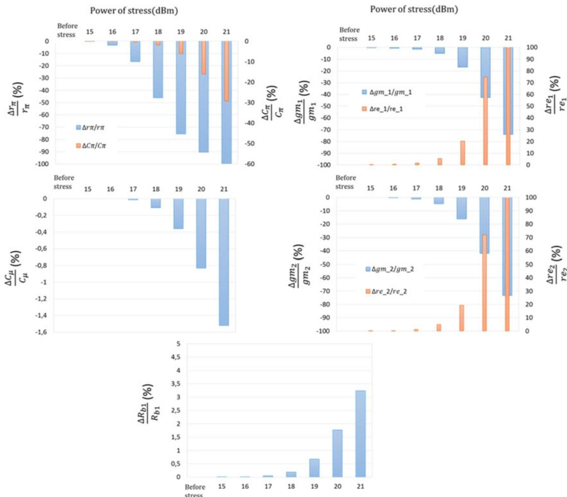
Fig. 14. LNA small-signal parameters degradation after 336 h of stress in function of RF input stress power.
