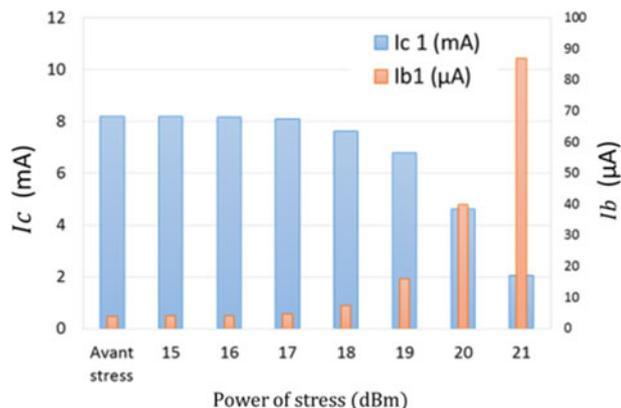
Fig. 15. DC currents after 336 h of stress in the function of RF input stress power.
