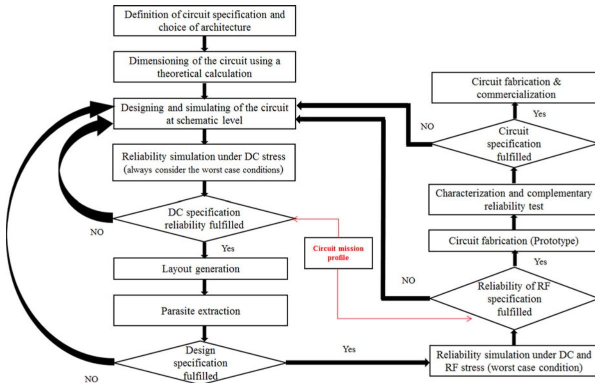
Fig. 16. Design flow aware circuit reliability: design steps illustration including reliability simulation.
