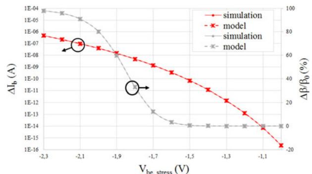
**Fig. 6.** Comparison of simulated  $\Delta I_b$  and  $\Delta\beta/\beta_0$  as a function of  $V_{be\_stress}$  based on RVBE degradation model (high-voltage SiGe NPN: after 10 years of stress at 40 °C).
