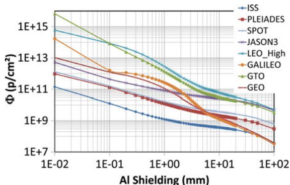
Fig. 2. Equivalent 80 MeV monoenergetic protons fluencies versus aluminum shield thickness for eight typical spatial missions. These fluencies are given for 1-year mission’s durations.
