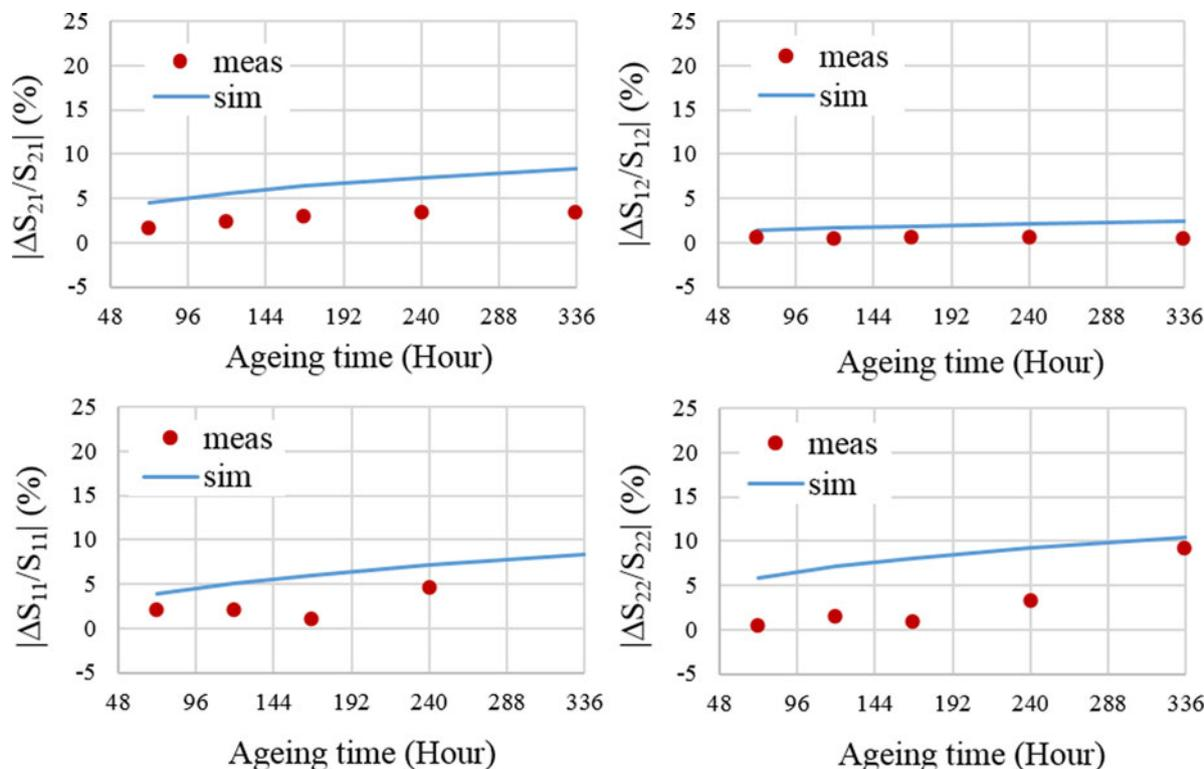
**Fig. 10.** Comparison between simulated and measured S-parameters degradation at 5.6 GHz after 336 h of 20 dBm stress:  $\Delta S_{ij}/S_{ij}$  is defined as the relative degradation.
