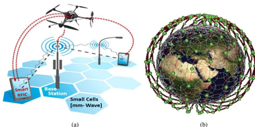
Fig. 1. Use of UAV systems in 5G as a relay between macro-cell base station and user equipment (a). Low earth orbit (LEO) in the perspectives of Internet Everywhere (b).
