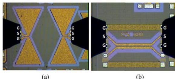
Fig. 3. Photomicrograph of the planar bowtie antenna (a) and the integrated CPS transmission line structures (b).
