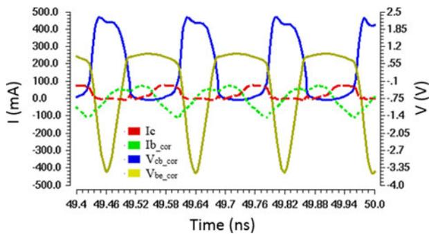
Fig. 8. AC collector-base voltage, AC base-emitter voltage, AC base current, and AC collector current of LNA during the application of RF power stress.
