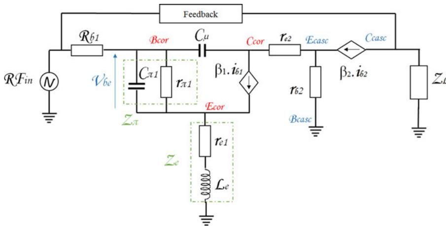
Fig. 13. Small-signal model of cascode LNA with feedback.
