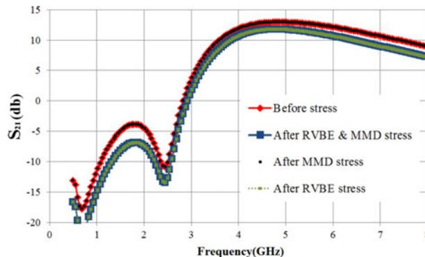
**Fig. 12.** Simulation of the contribution of MM and RVBE degradation mechanisms to the LNA gain shift after 336 h of 20 dBm stress.
