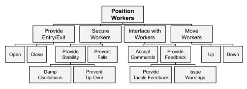
Figure 2: Example of function tree in context of articulating-boom construction lift
