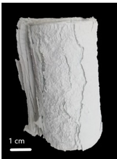
Figure 2 Lead white produced after one month of exposure of lead to vinegar and horse manure (setup 4). The corresponding diffractogram is presented in Figure 3b.
