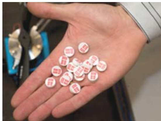
Figure 3. Pellets of Mg(NH_3)_6Cl_2 , a carrier for ammonia. The pellets hold NH_3 at nearly its density in liquid ammonia, but at a vapor pressure of only 2 mbar; there is no significant release of ammonia to the environment and the pellets can be handled safely. The pellets are charged at room temperature and release ammonia above ~100°C. After Reference 31.
