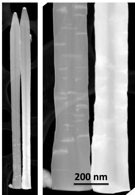
Figure 3. STEM images of the core-shell NWs show planar defects in the bottom half of the NWs.
