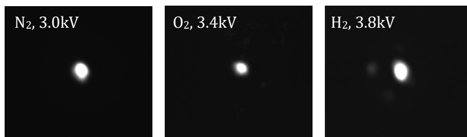
Figure 1. A typical W(111) SAT prepared by annealing in presence of nitrogen. Stable ion beams were generated using (a) nitrogen, (b) oxygen, and (c) hydrogen.
