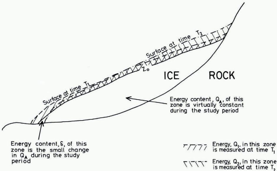
Fig. 1. Longitudinal section of a valley glacier showing zones with their associated energy content.
