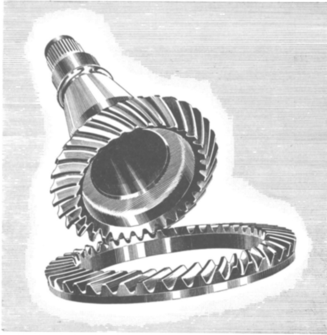
ENV spiral bevel gears used in Westland S 55 main rotor drive
