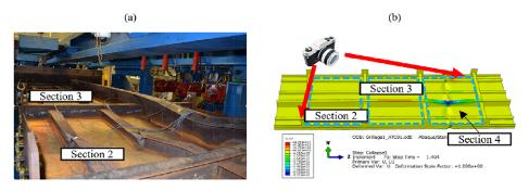
*Figure 10.* Failure mechanism and location comparison between (a) the physical test (reprinted from Nahshon et al. (2021)) and (b) the finite element model simulation. Camera in (b) shows photographer location in (a).
