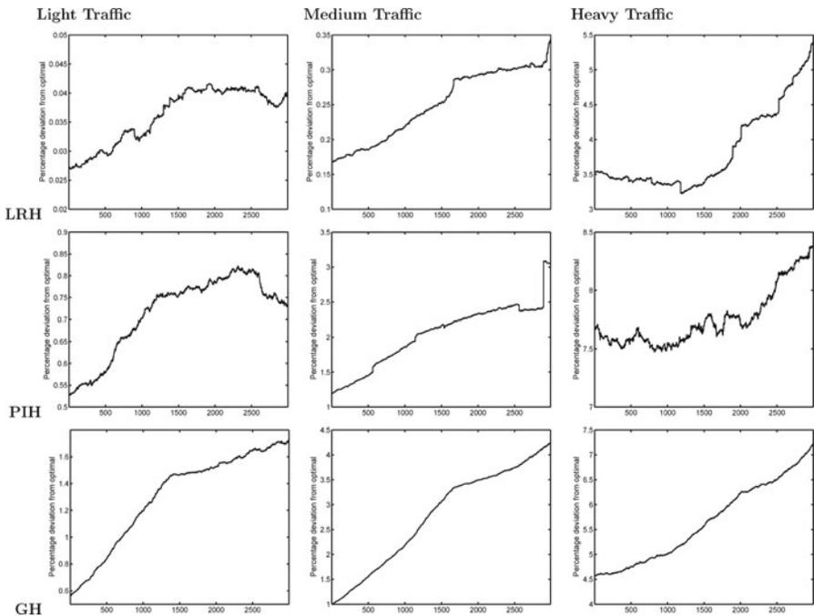
**FIGURE 1.** Moving average plots of percentage deviations of heuristics from the optimal with respect to the number of scenarios that are ordered according to the increasing heterogeneity index of dedicated load  $\Phi$ .
